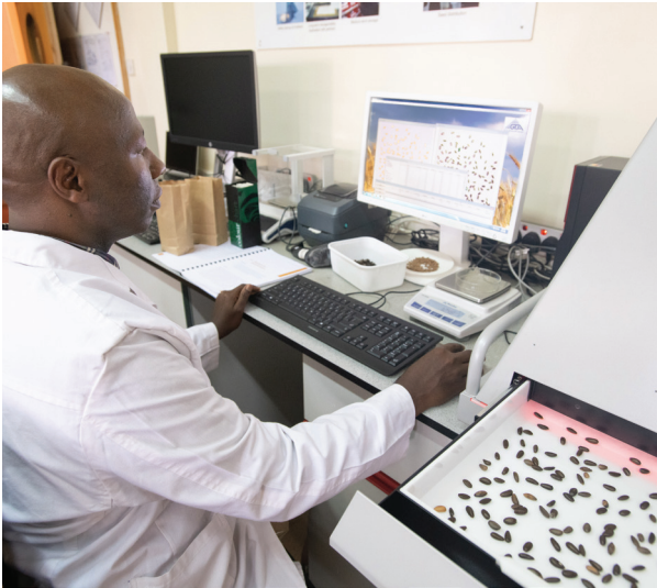
Simon Kang'ethe (ICRAF) conducts seed characterization of Annona squamosa using the Marvin5 seed analyser. Photo: Michael Major/Crop Trust
